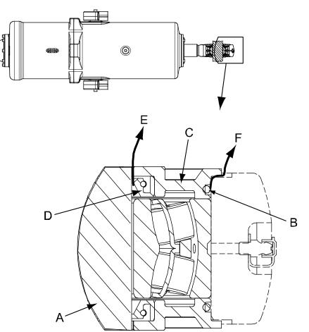
Check the o-rings in the front ear of the balancing device for leaks, as shown and detailed below.
