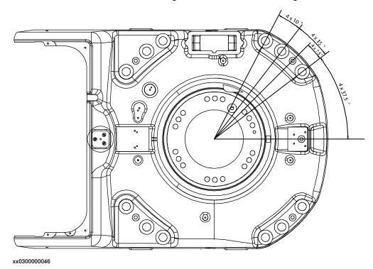
This illustration shows the hole configuration used when securing the robot.
