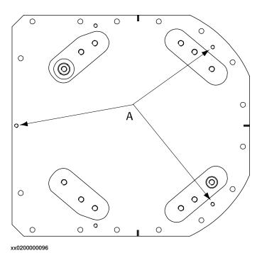
A Attachment holes for lifting eyes (x3)
