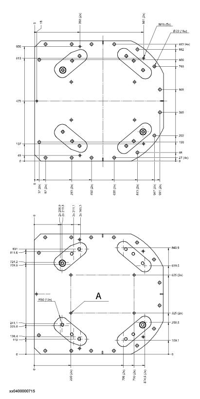
A Four holes for alternative clamping, 4x Ø18
