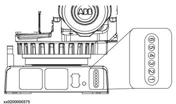
Internal brake release unit with push buttons, located on the robot base
