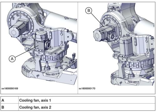
2.3.10 Installation of cooling fan for motors (option) *Continued*
