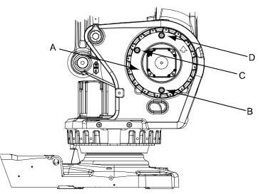
The figure shows position of gearbox, axis 3.
