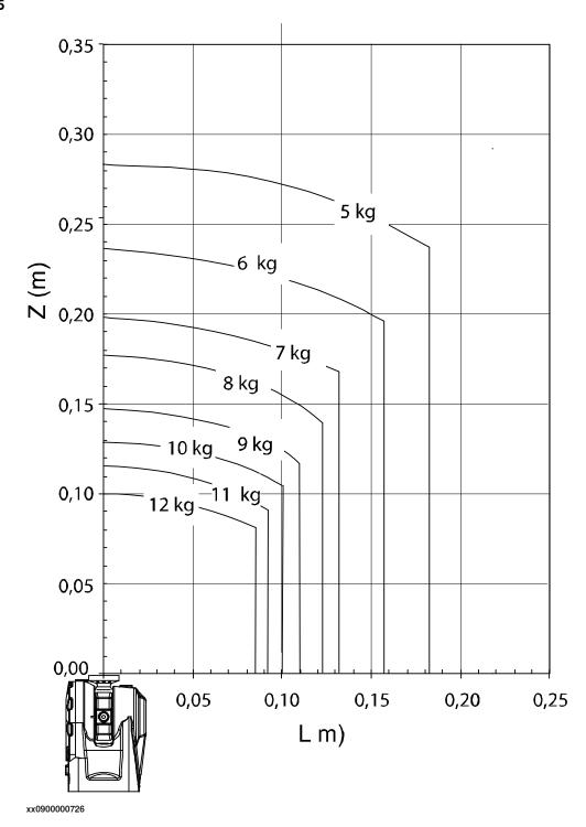
Extra load of 15 kg at the upper arm housing and 1 kg at wrist included in the load diagram.
