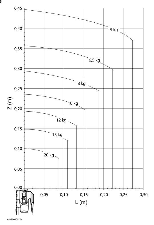
Extra load of 10 kg at the upper arm housing and 1 kg at wrist included in the load diagram.
