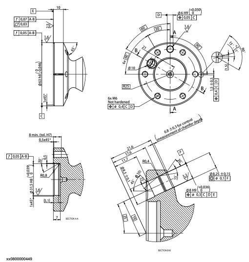
For fastening of gripper tool flange to Robot tool flange every one of the screw holes for 6 screws, quality class 12.9 shall be used. Min. 10 mm used thread length.
