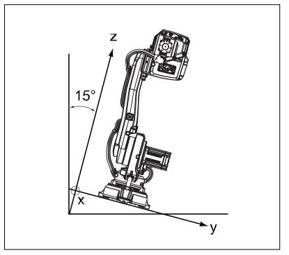
Examples of mounting angles tilted around the X axis (Gravity Alpha)
