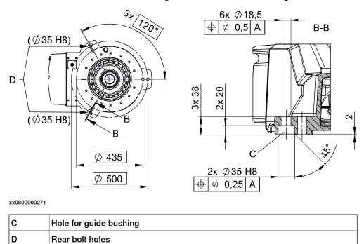
The illustration shows the hole configuration used when securing the robot.
