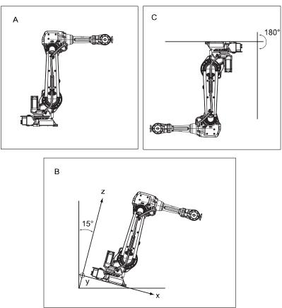
Examples of mounting angles tilted around the Y axis (Gravity Beta)
