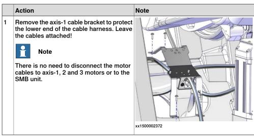
Preparations of axis-3 before lifting away the lower arm complete
