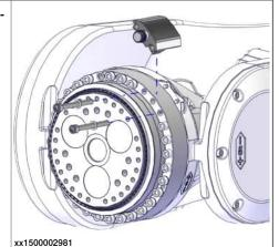
Unscrew the attachment screws that secure the axis-6 gearbox.
