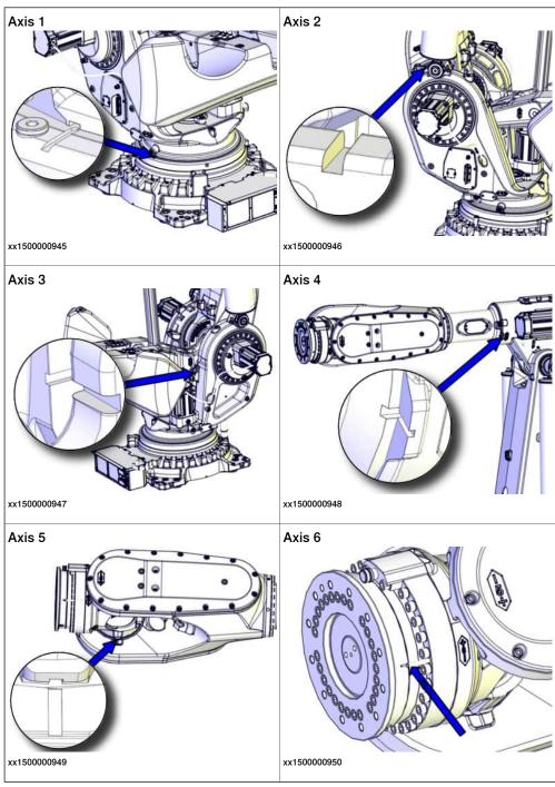
5.2.2 Calibration movement directions for all axes
