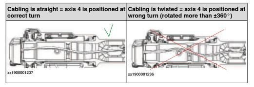
Step 1 - Manually running the manipulator to the synchronization position
