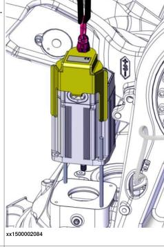
10 Disconnect the brake release tool / 24 VDC power supply.
