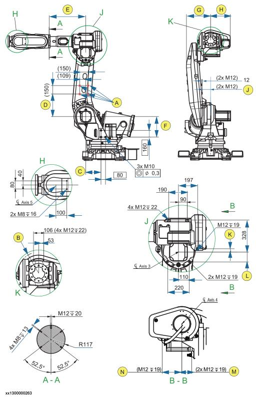
A Allowed position for attachment holes, M12 through. Be careful not to touch the cables when drilling.
