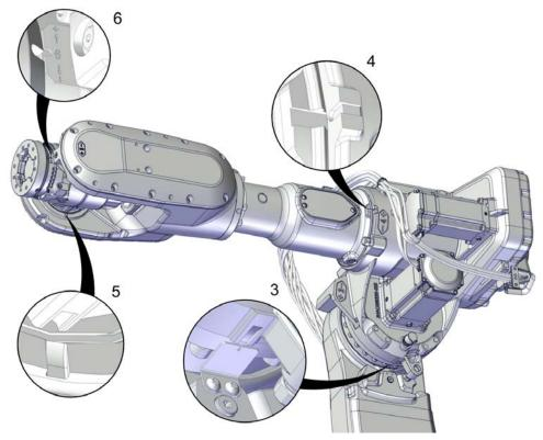
2.4.2.2 Calibration movement directions for all axes
