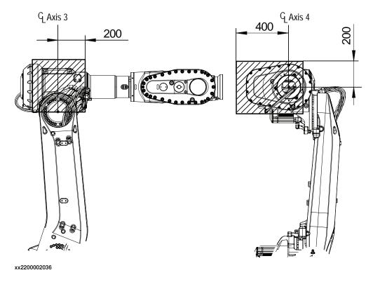
2.2 Fitting equipment on the robot (robot dimensions)
