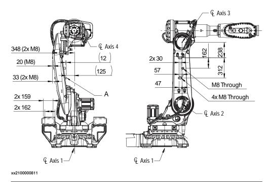
A Allowed positions for attachment holes. 4x M12 through. Avoid damaging cables when drilling.
