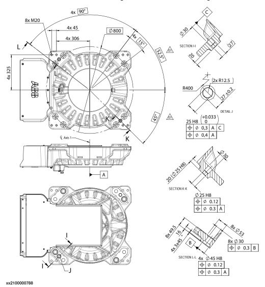
2.3.1 Installing a base plate
