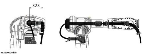
Spotwelding option 3325-51/52/52/61/62/63 (Base to axis 3) + Option 3326-50/51/52/52/61/62/63 (Axis 3 to axis 6)
