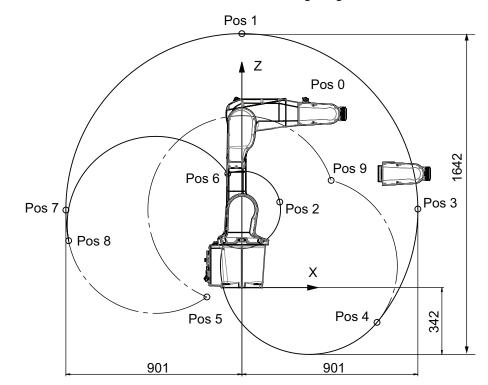
IRB 1200-5/0.9 Working range, positions at wrist center and angle of axes 2 and 3 The illustration shows the unrestricted working range of the robot.
