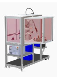
The arc welding FlexTrainer is designed to maximize the required training needs to master robotic welding programming, electrical service, mechanical maintenance, and off-line/on-line software packages. All educational software packages are included with the robot.
