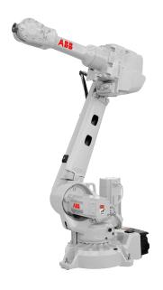
The IRB 2600 is the second model in the sharp generation range with enhanced and new capabilities. It is a compact robot with a high payload capacity. The design has been optimized for targeted applications like arc welding, material handling and machine tending. The IRB 2600 is available in three variants, with options for floor, wall, shelf, tilted or inverted mounting configurations.
