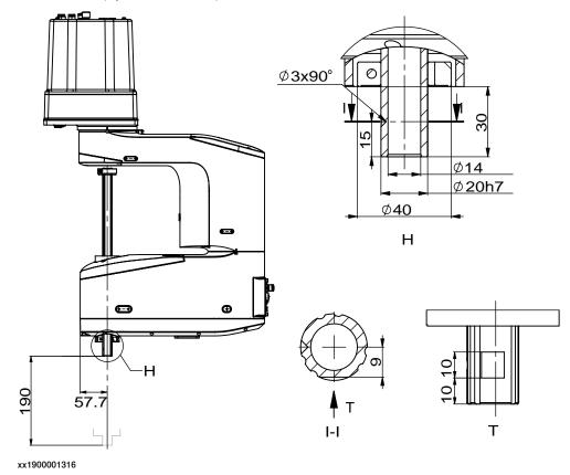
3.3.7 Fitting equipment on the robot (robot dimensions)
