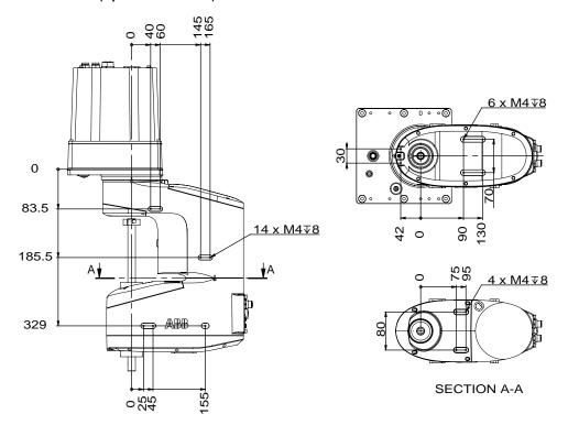
3.3.7 Fitting equipment on the robot (robot dimensions)
