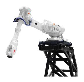
The IRB 6650S is the shelf robot form of the Power Robot family which offers a unique working envelope. It is capable of a full vertical and horizontal stroke motion, as well as an increased forward and downward reach. This combination offers new possibilities to robot functions in numerous application areas.
