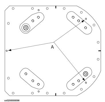
A Attachment holes for lifting eyes (x3)
