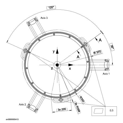
The three support points of the manipulator base box shall be mounted against three flat surfaces within the specification above. Shims is used if necessary.
