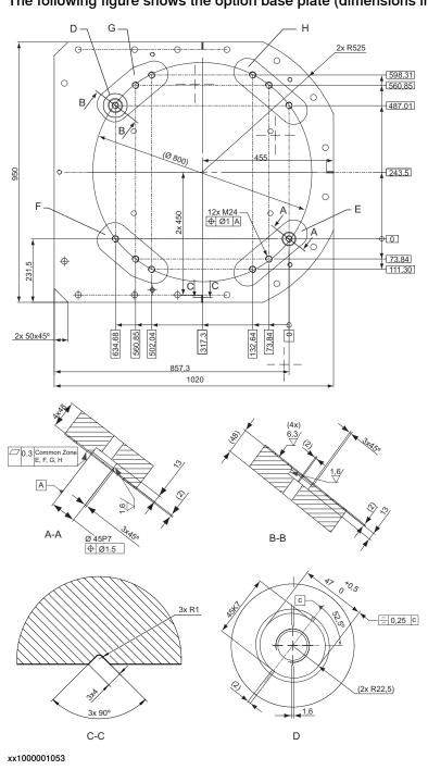
The following figure shows the option base plate (dimensions in mm).
