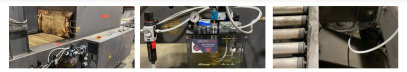
A customer wanted to eliminate the hassle of brushing oil onto chains. The goal was to reduce the amount of manpower needed to lubricate the machine. GreasePoint and the PennAir Field Service teams installed the system before the next plant production run. The installation will help improve component life, machine accuracy, safety, production, lube efficiency, and reduce waste.
