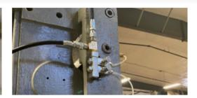
A customer bought a new machine that needed major upgrades and had three more on the way. GreasePoint and the PennAir Field Service team were able to install the lubrication pump in one day. This install will save the operator from oiling the machine each morning. The pump will help improve component life, machine accuracy, safety, production, lube efficiency, and reduce waste.
