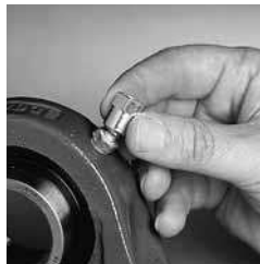
2. Place a Zerk-Lock onto the fitting
