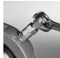
4. Then thread a Quicklinc completely into the Zerk-Lock
