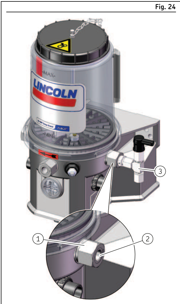
Replacing pump element and pressure limiting valve
